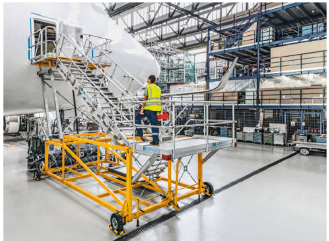
Special maintenance steps with intermediate platform for passenger access
