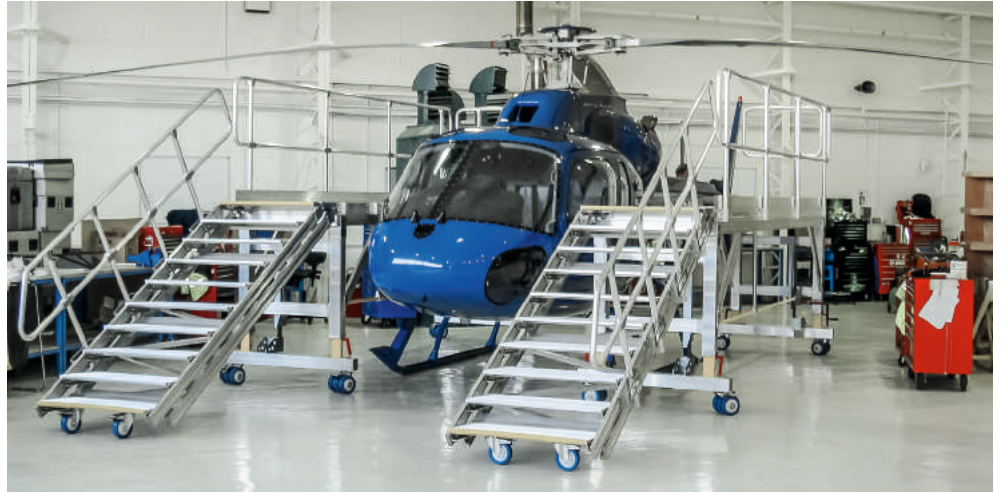
Maintenance platform for EC 145; height-adjustable
