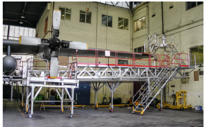
Wing dock for C130 Hercules with fixed height
