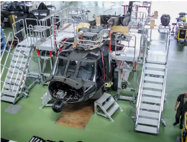
Dock system for Black Hawk; height-adjustable
