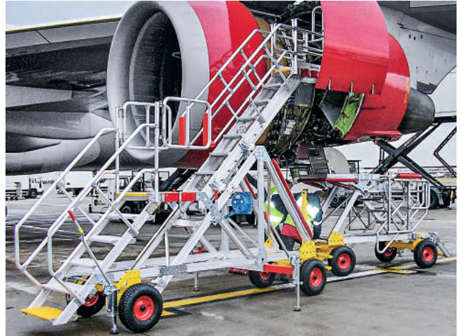
UCAS (Under Cowling Access Step)
