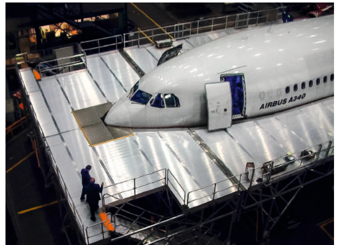
Fixed-height dock for A330/A340 with foldable passenger access platform
