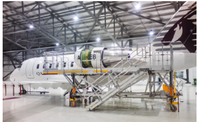
Height-adjustable engine dock for CL300,605, Global Express
