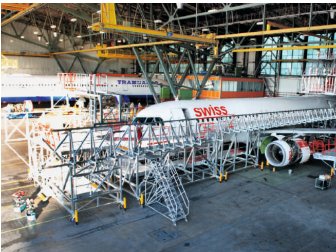
Fixed-height dock with 2 levels for A320 family
