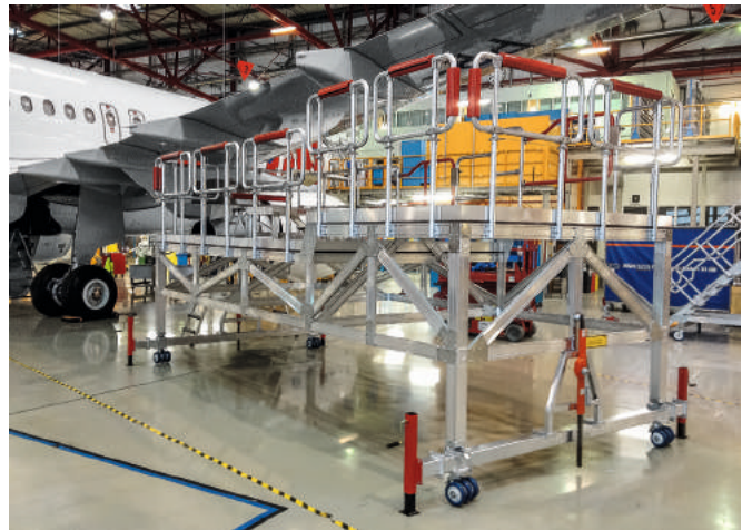
Maintenance platform for flap rigging of A320
