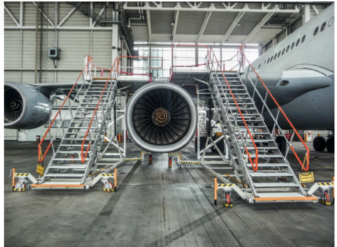
Set of height-adjustable steps for pylon and precooler access on A340 and B747
