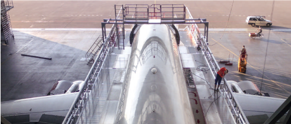
Fuselage dock including bridge; fixed height with 2 levels for A320 Family
