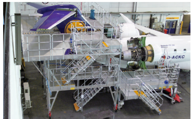
Height-adjustable tail and engine dock for Bombardier CRJ900
