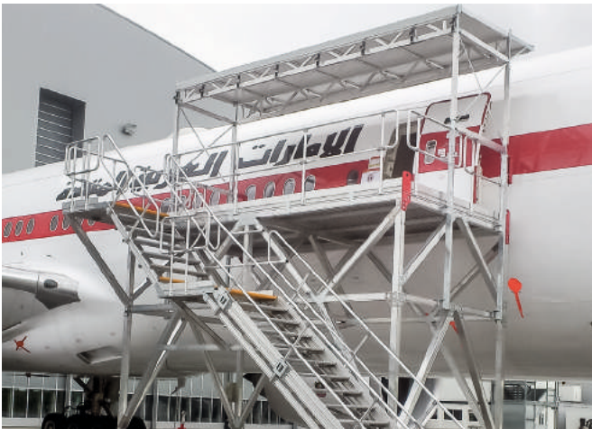
Maintenance platform with detachable cover
