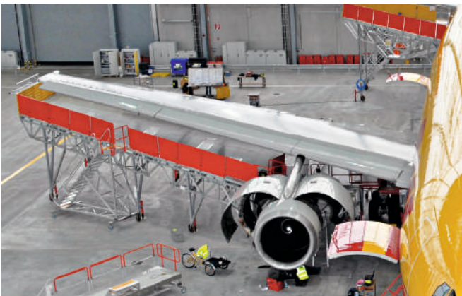
Two-piece wing dock for A300 with fixed height and media technology
