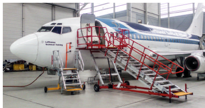
Passenger door access for B737; height-adjustable
